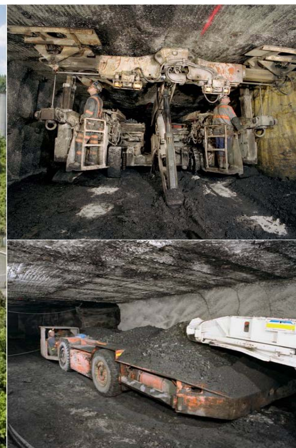
> Underground operations : roof bolter and shuttle car
